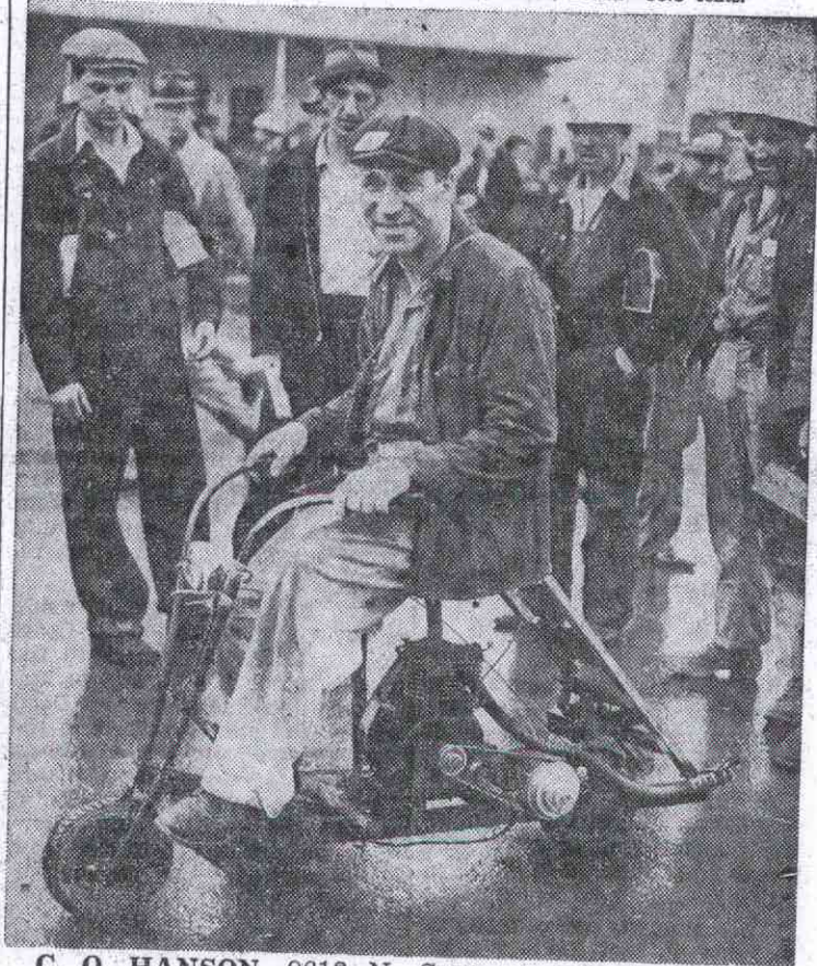
C. O. HANSON, 9613 N. Syracuse street, Oregon Shipbuilding corporation worker, has solved his own transportation problem by building himself a motor bike out of odds and ends. The motor once ran a washing machine, the wheels and pulleys came from a local department store, and the headlight was intended for a bicycle.
