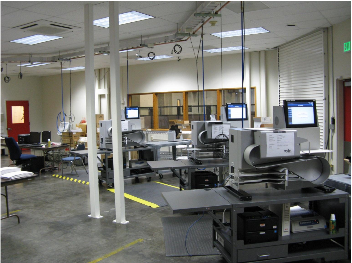
Photograph 10: DS850 Testing Setup
