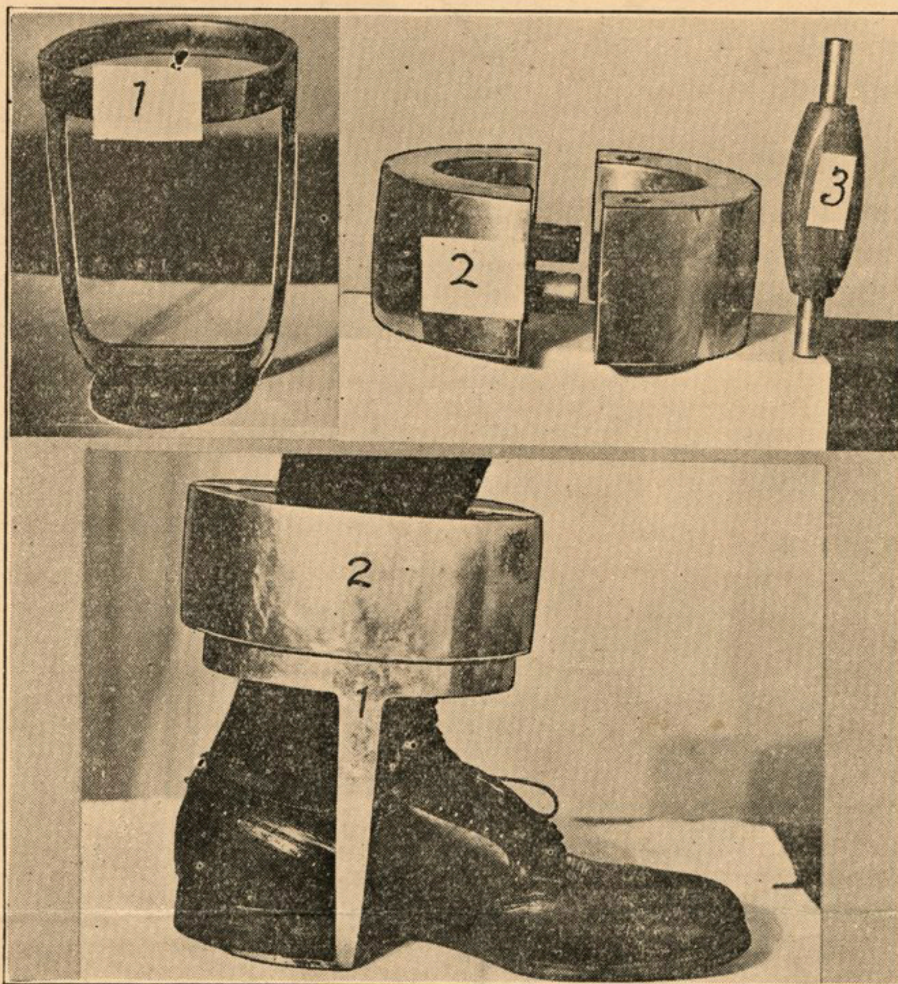
FIG. 1: Lower portion that screws on heel of shoe and supports 15-pound weight.
